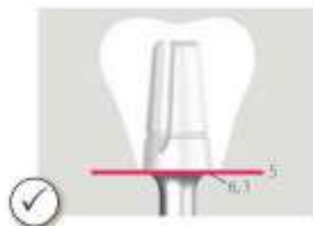
Fig. 3 The crown margin (6) will be the same level as the lower border of the abutment head (1) if the abutment head sits on the mucosa line (5).
